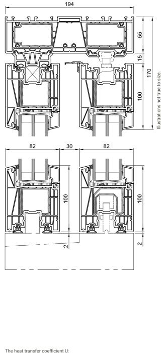
The lower the U-Value, the less the heat loss in winter and the permeability of heat in summer. U, (frame) refers to the insulation value of the frame-sash combination while  $U_w$  (window) refers to the overall structure including the glazing.
